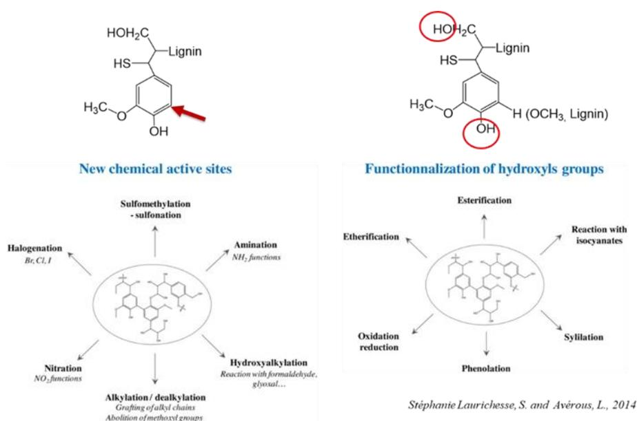
**Figure 1.11.** Illustration of two main approaches in the chemical modification of lignin macromolecule: through the functionalization of hydroxyl groups and the introduction of new chemical sites into aromatic ring of phenylpropanoid unit (PPU).
