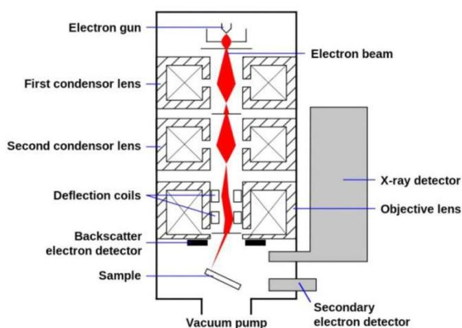
**Figure 3.10.** Schematic illustration of SEM (Alqaheem and Alomair, 2020).
