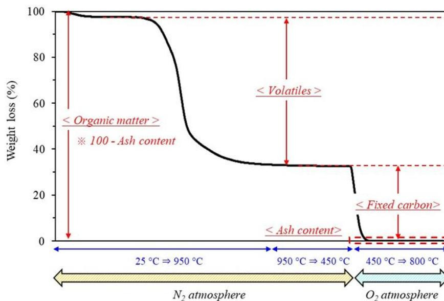
**Figure 3.6.** Thermogravimetric analysis of lignin (adapted from Tagami, 2018).
