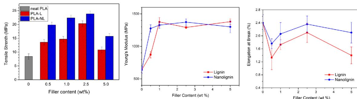
**Figure 2.15.** Mechanical properties of PLA/L and PLA/NL (Makri et al., 2022).
