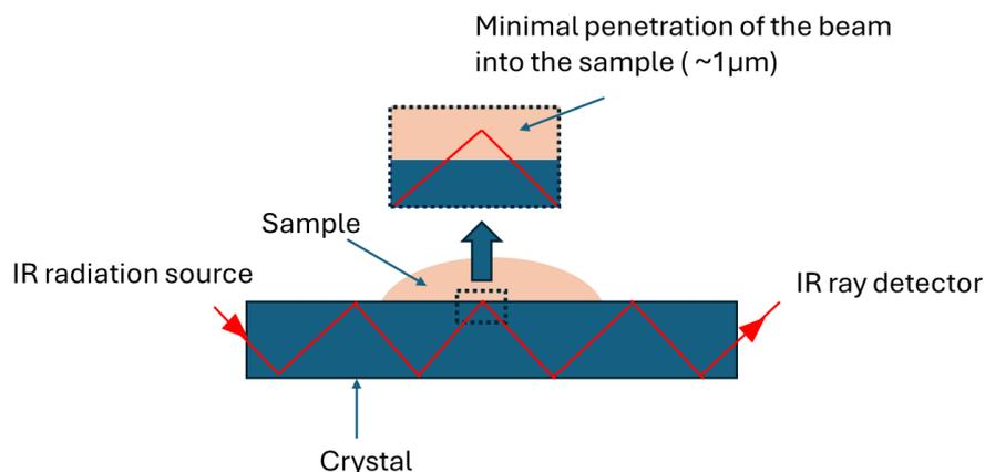
**Figure 3.1.** The phenomenon of total internal reflection inside the ATR attachment crystal.
