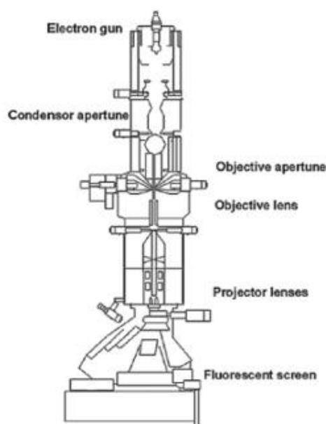
**Figure 3.11.** Schematic illustration of TEM (Alqaheem and Alomair, 2020).
