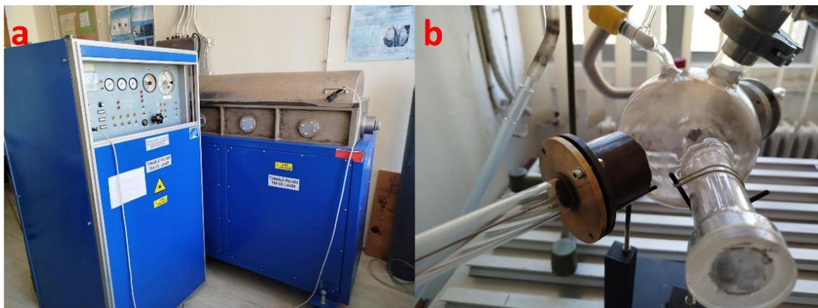
**Figure 3.14.** CO<sub>2</sub> laser and its control board (a) and glass reactor (b).
