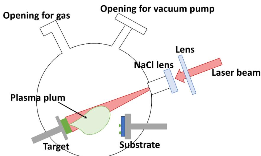
**Figure 3.13.** Schematic illustration of the reactor for PLA.
