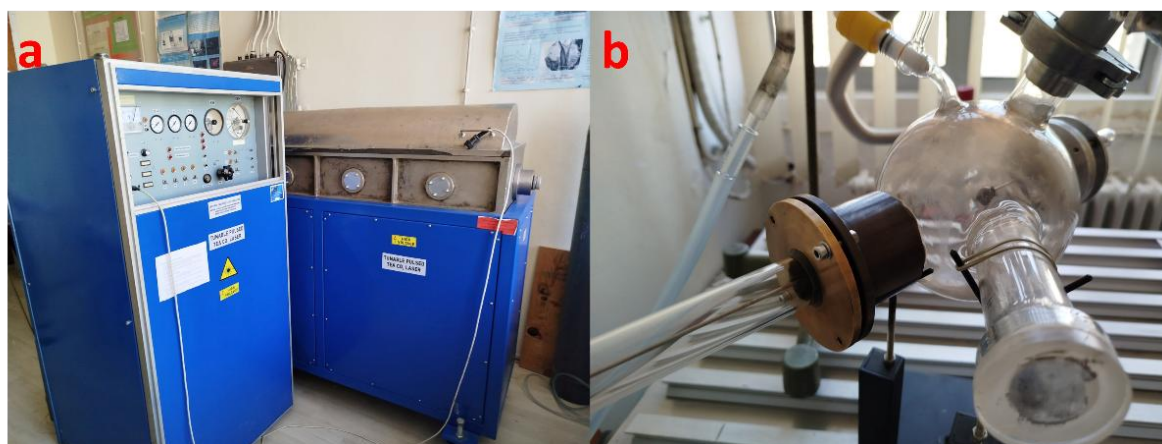
Figure 3.14. CO 2 laser and its control board (a) and glass reactor (b).
