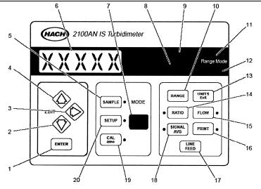
Fig. 7. Laboratory Turbidimeter 2100AN IS
