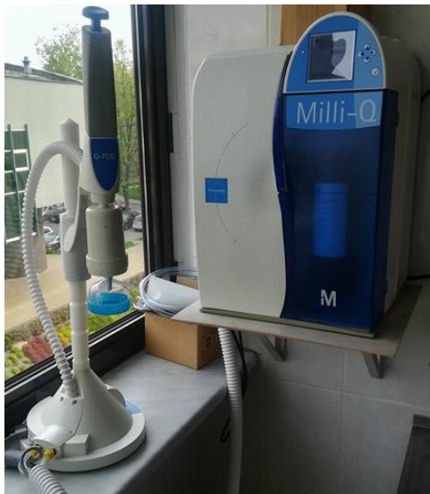
system for ultrapure water production
