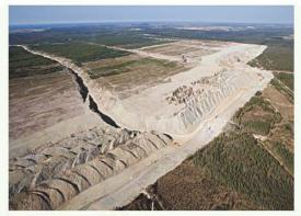
Figure. Open-cast oil shale mine
