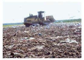
Figure 10.19. Compaction of solid waste at the Getliņi sanitary landfill in Latvia
