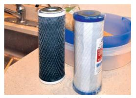
Figure 10.12. Personal water filter after use (left) compared to a new one (right)
