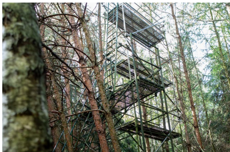
Platform enabling pine needle collection and analysis at various heights.
