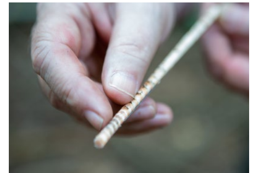
Retrieving tree bore with a Pressler drill allows trees' age to be determined and to calculate the dynamics of their annual growth in thickness.
