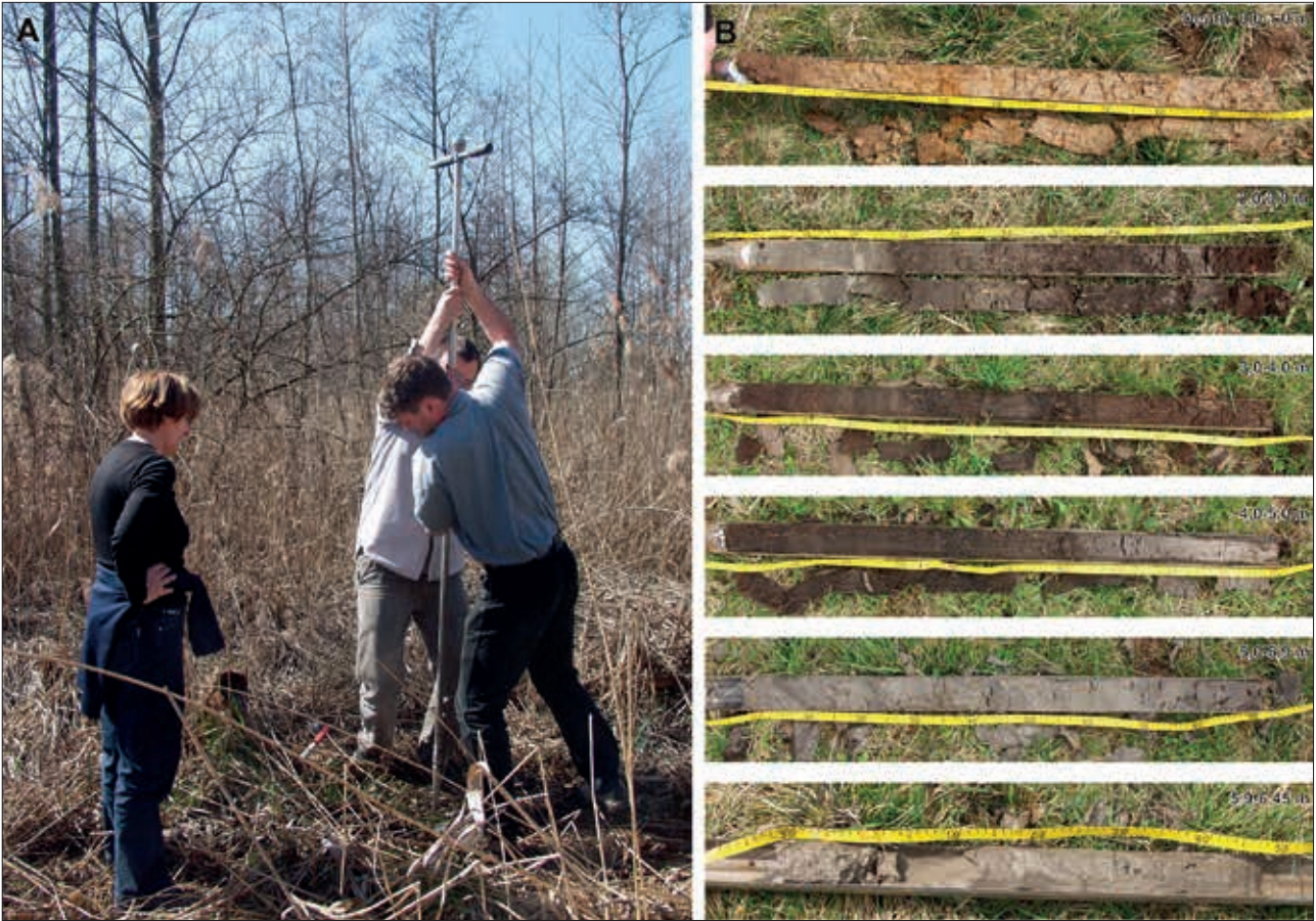
Figure 2.15. Coring in the floor of the Opatówka Valley (A) and core samples obtained in 2007. Photograph by M. Łanczont.
